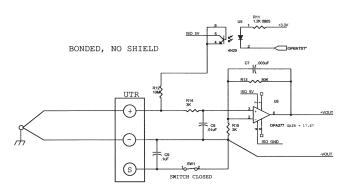
FIGURE 4.8 - UNTERMINATED PROBE THERMOCOUPLE
