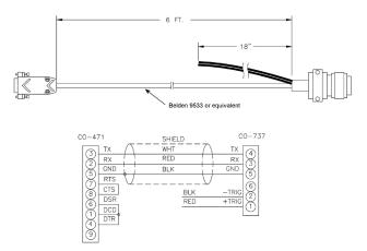
FIGURE 3.1 - SERIAL COMMUNICATION/TRIGGER CABLE
