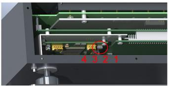
FIGURE 3.6 - DIP SWITCHES
