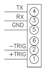
FIGURE 3.5 - TRIGGER WIRING
