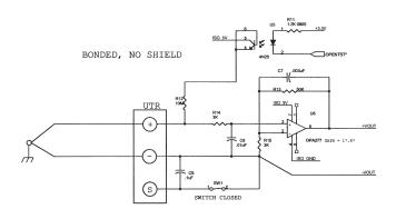
FIGURE 4.4 - BONDED THERMOCOUPLE, NO SHIELD
